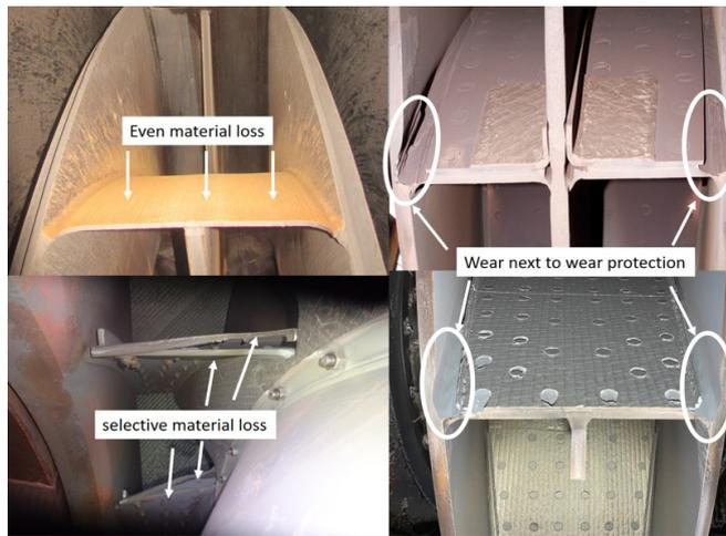
Figure 1. Different kinds of wear on a radial impeller.
