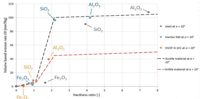
Figure 2. Volume based erosion rate for a  $20^\circ$  impingement angle.
