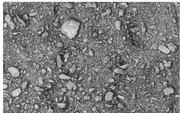
Figure 4. Example of particles a centrifugal fan is exposed to.
