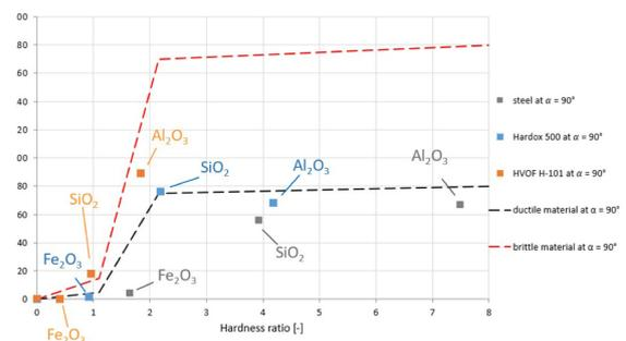
Figure 3. Volume based erosion rate for a  $90^\circ$  impingement angle.
