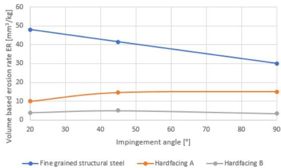
**Figure 5. Volume based erosion rate for a specific set of erosive particles.**
